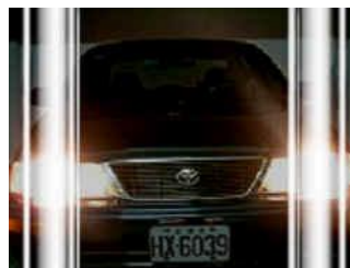
Poor view due to smear
